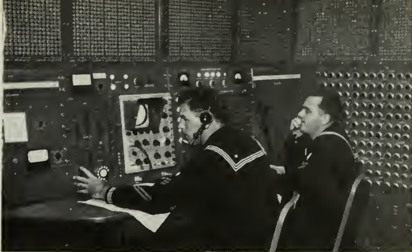
IT'S N.E.W.S.—Whitehat experts man controls of Navy's Electronic Warfare Simulator at Naval War College. NEWS can simulate naval battle conditions.
